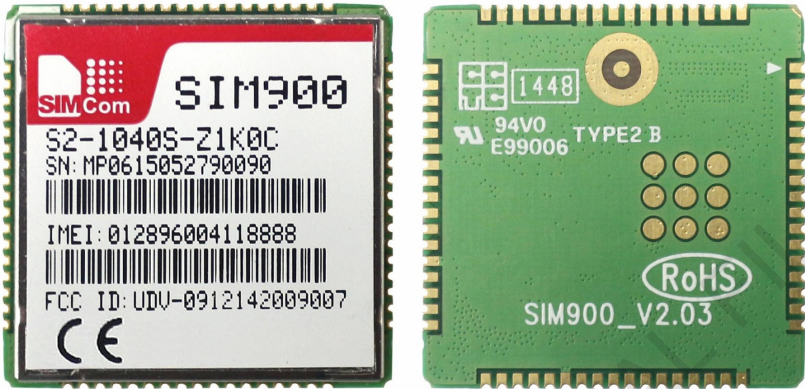
Figure 7: SIM900 Top, bottom and side view
