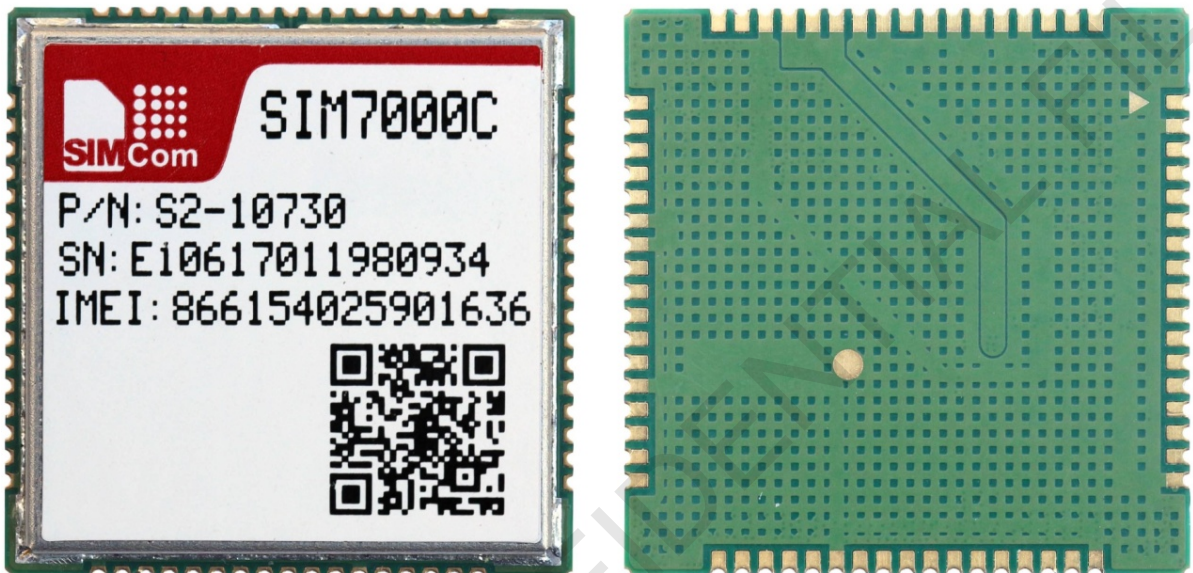
Figure 5: Top and bottom view of SIM7000
